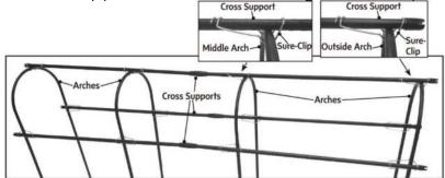
Tip: When attaching a cross support using the sure-clips, remember that the support should always be on the outside of the arches and that the curved part of the clips will always be facing towards the inside of the pea tunnel.
