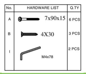
1. Connect the arms of the bench to the seat using screws (A) and the allan key.
